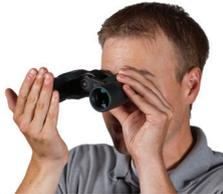
2. Adjust the diopter. Close your left eye or cover the left objective lens with your hand and rotate the diopter ring until the object is in focus.
