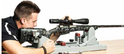
Visually bore sighting a rifle scope.
