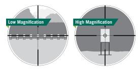
**Note:** The Diamondback® Tactical 4-12x40 riflescope's reticle is calibrated to 12x. For a hashmark's value to be true, it would need to be used on 12x.
